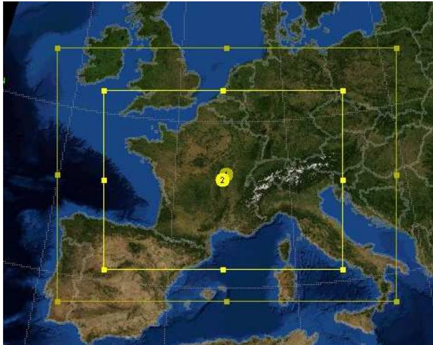
*Fig. 2: Multi-nesting process with two domains of the anemos wind atlas France 3 km. Domain 1 with 15 x 15 km<sup>2</sup> and domain 2 (Nest) with 3 x 3 km<sup>2</sup>.*
