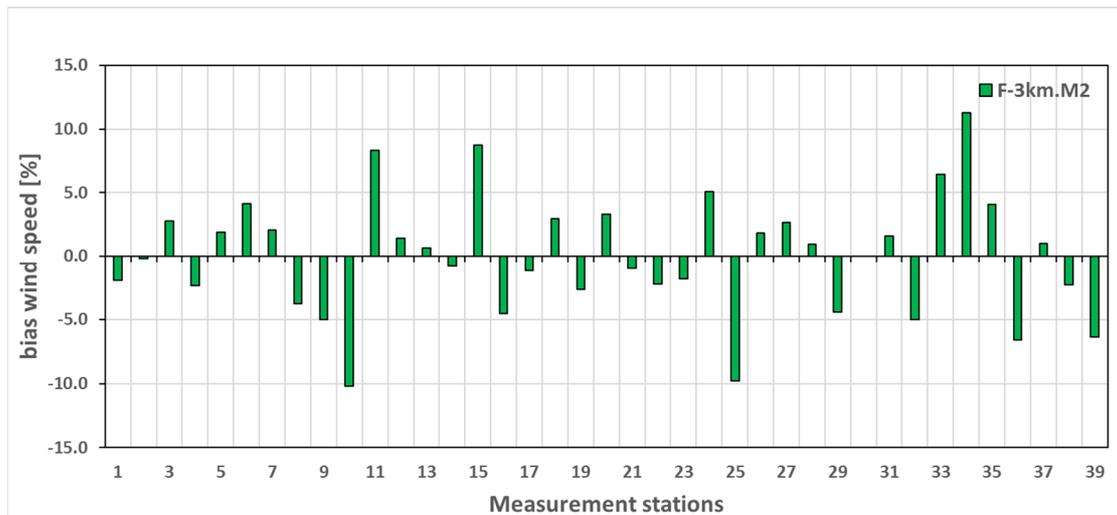
Fig. 4: Bias in mean wind speed between 39 internal wind measurements and the F-3km.M2 wind atlas (green). The measurement height is between 40 - 120 m.
